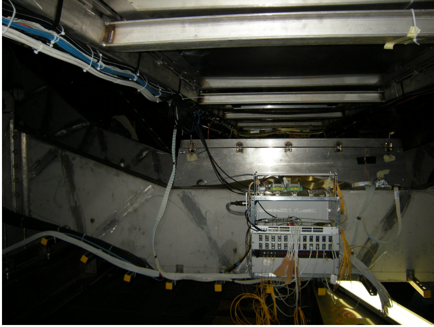
Figure 4: PHOS modules in the pit P2. Disposition of the trigger Fan-Out panel is just before PHOS.
